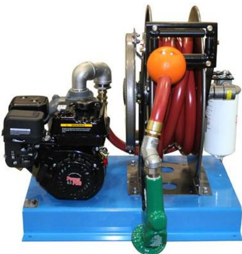
**1-1/2" Units** also include Cimtek 1-1/2" 60 GPM fuel filter with 2-30 micron Hydrosorb elements, 35' of 1-1/2" fuel transfer hose and Husky 1690 1-1/2" high flow automatic nozzle. All units are mounted on steel base plates (*powder-coat finish*).
